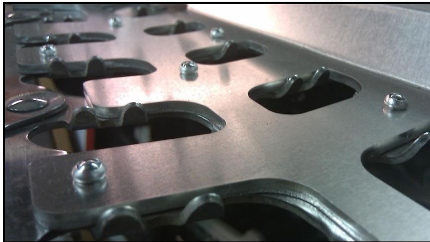
Figure 6 – Rivet positions following installation on the running board floor
