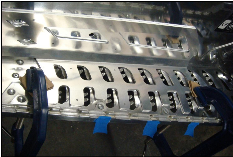
Figure 4 – Properly seat support against tunnel and lightly clamp in place
