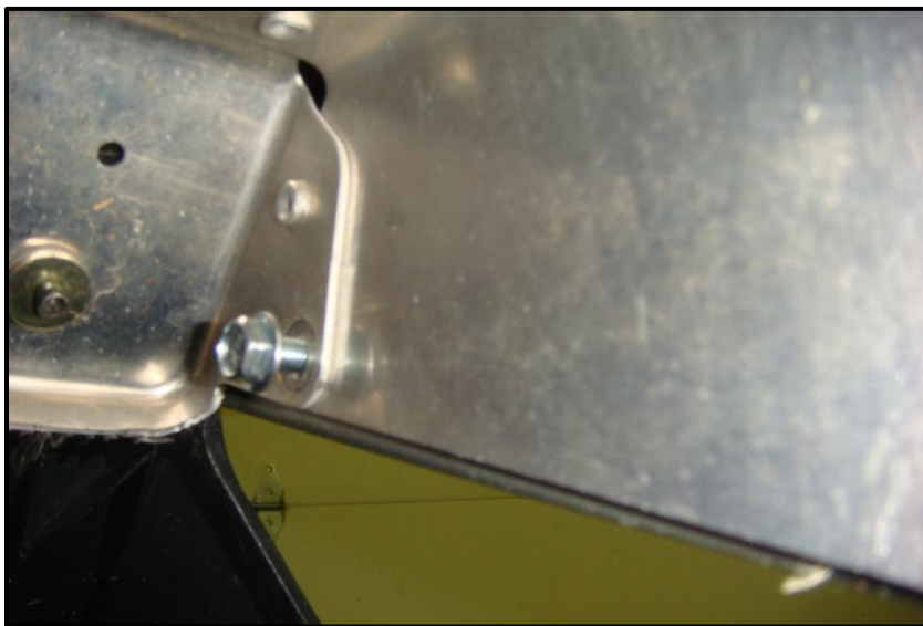
Figure 3 –New rear bolt (4) - (LH side shown)
