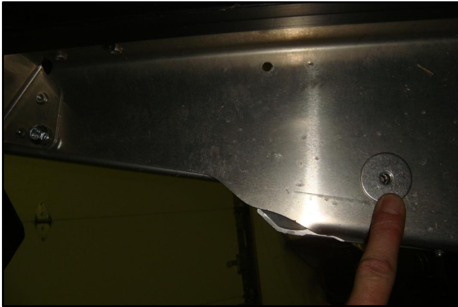
Figure 4 –Spacer located over front mounting hole. (LH side shown)
