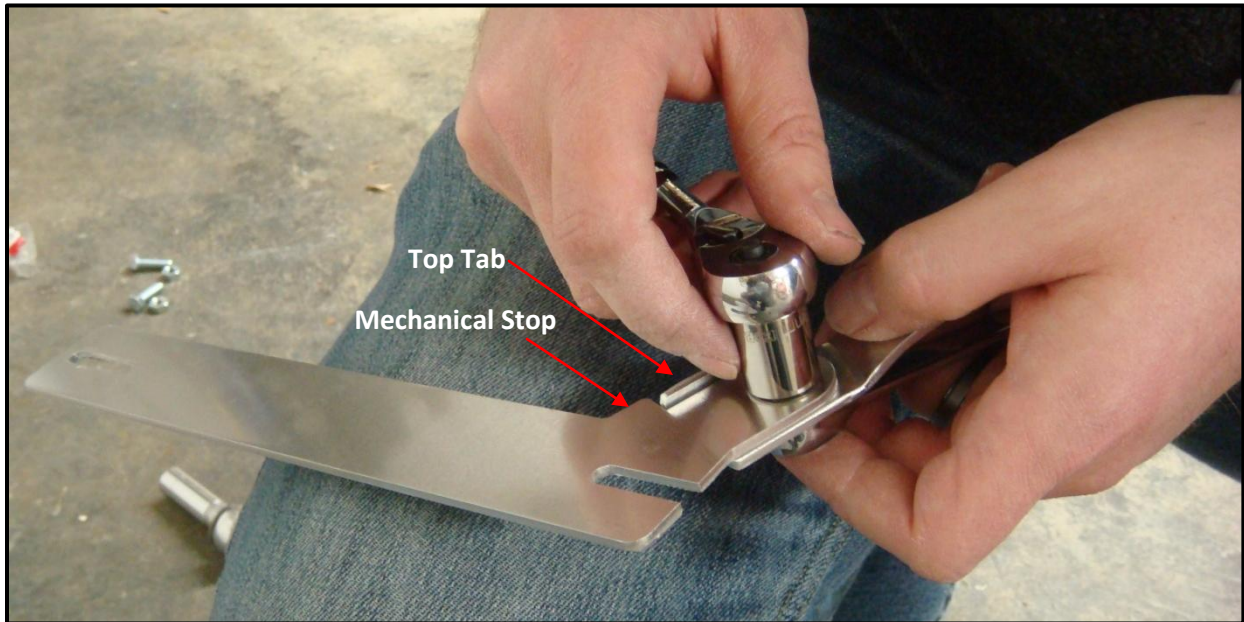
Figure 1 –Bolt pivot arm to mounting base
