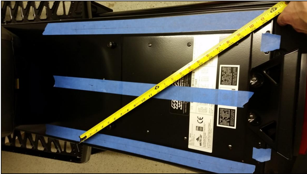
Figure 7 – Check diagonal measurements to ensure hole pattern is square
