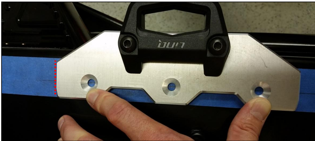
Figure 6 – Mark the front edge of the Adapta-Link in the desired location
