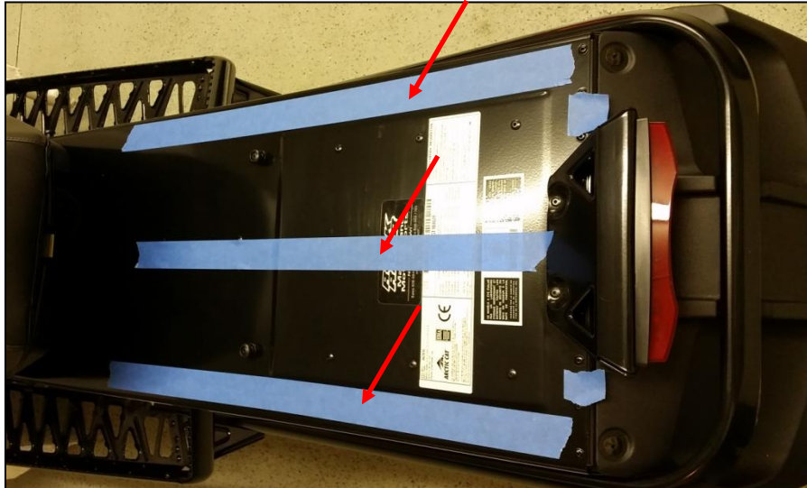
Figure 1 – Place tape on tunnel centerline and outer edges (appx 12 5/8" on center)
