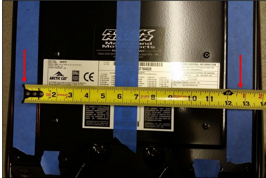
Figure 3 – Find tunnel centerline and mark
